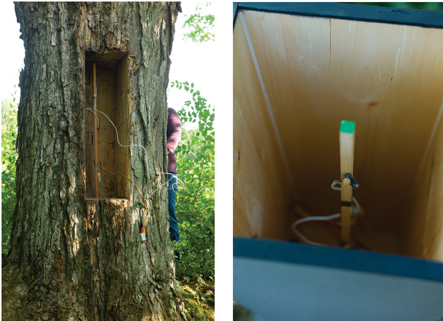
Fig. 2 Views of the cavities inside the maple tree and the wooden box. One sees the temperature sensor in each cavity, positioned 25 inches (64 cm) above the floor.
